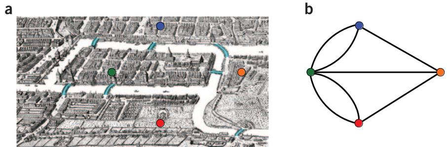
**Figure 1** Bridges of Königsberg problem. (a) A map of old Königsberg, in which each area of the city is labeled with a different color point. (b) The Königsberg Bridge graph, formed by representing each of four land areas as a node and each of the city's seven bridges as an edge.
