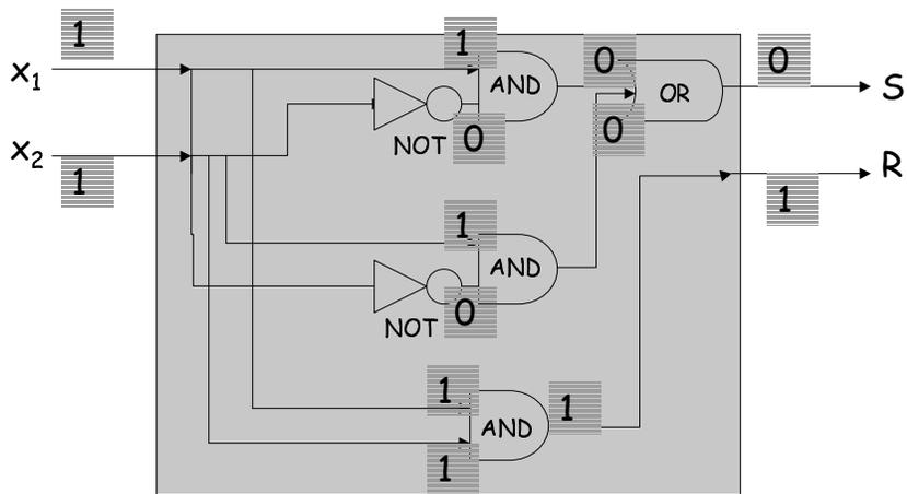
$$S = (x_1 \text{ AND NOT}(x_2)) \text{ OR } (x_2 \text{ AND NOT}(x_1))$$
