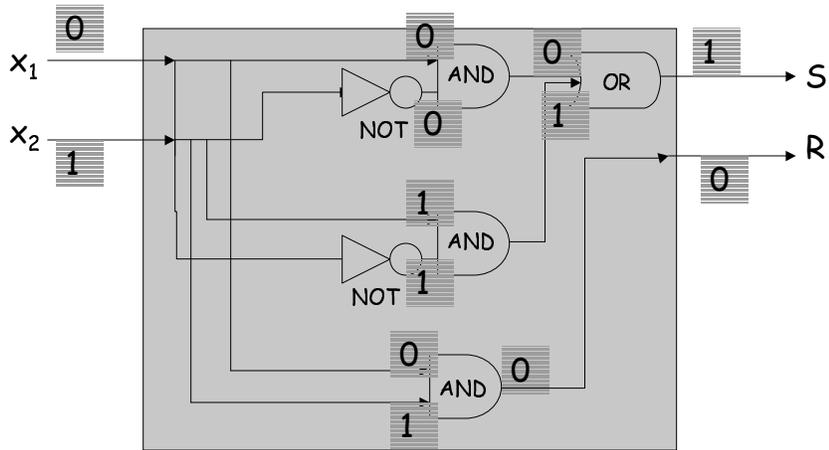
$$S = (x_1 \text{ AND } \text{NOT}(x_2)) \text{ OR } (x_2 \text{ AND } \text{NOT}(x_1))$$
