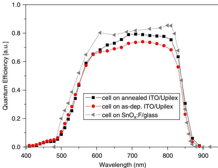
Fig. 5. A comparison of the quantum efficiencies of flexible solar cells with a cell on glass (12.5% efficiency). Efficiencies of the cells on as-deposited ITO and annealed-ITO are 8.5% and 11.4%, respectively, (AM 1.5).
