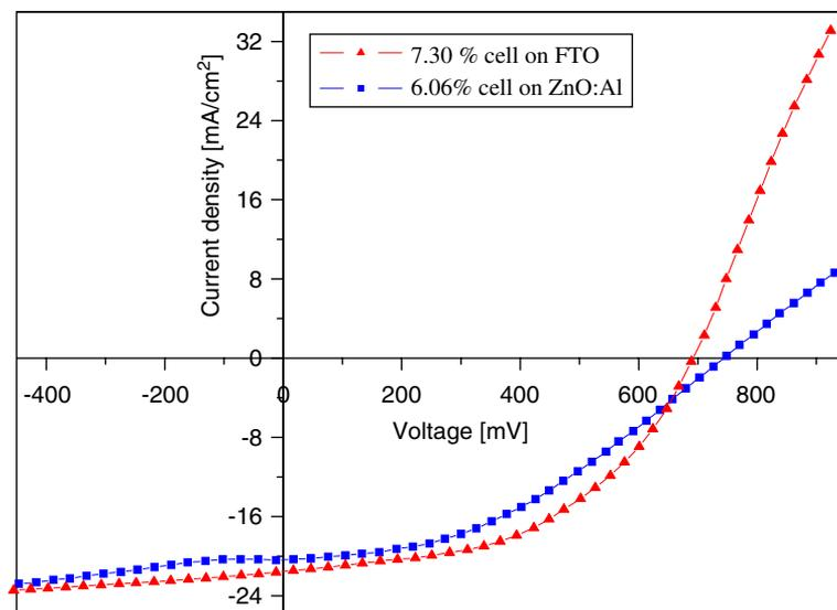
Fig. 8.  $I$ - $V$  performance of flexible solar cells in substrate configuration with FTO and ZnO:Al as front contact under AM1.5 illumination.
