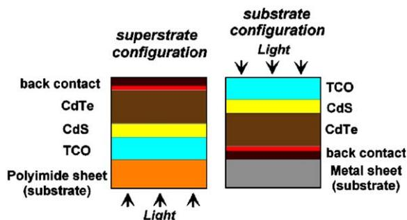
Fig. 2. Schematics of superstrate (left) and substrate configuration (right) solar cells, respectively, on polyimide and on metal sheets.
