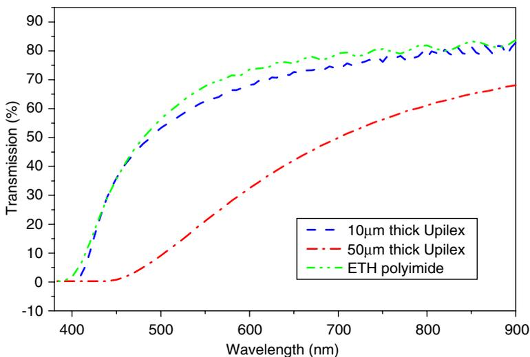
Fig. 3. Transmission spectra of different polyimide films, transparency is strongly dependent on the polyimide thickness.
