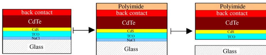
Fig. 6. Schematics of the flexible cell process in substrate configuration: after the polyimide is deposited on top, the cell is rinsed in water (in order to dissolve NaCl) and lifted-off from the glass.
