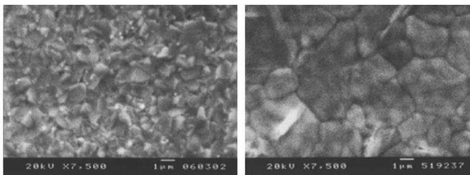
Fig. 7. As-deposited (left) and CdCl<sub>2</sub> treated (right) CdTe layers on CdS/TCO/NaCl stacks, the morphology is similar to the one shown in Fig. 4.
