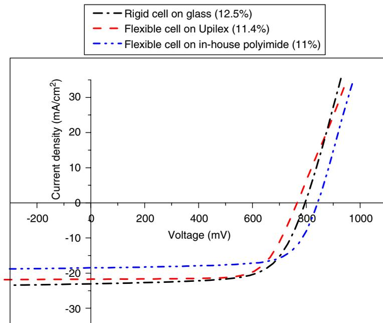
Fig. 1.  $I$ - $V$  curves of a standard CdTe solar cell on glass with 12.5% efficiency, on Upilex<sup>TM</sup> with 11.4% efficiency, and on in-house processed polyimide with 11% efficiency under AM1.5 illumination.
