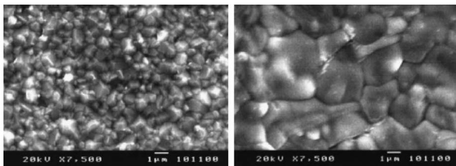
Fig. 4. As-deposited (left) and  $\text{CdCl}_2$  treated (right)  $\text{CdTe/CdS/TCO}$  layers on polyimide, the layers are compact and crack-free.
