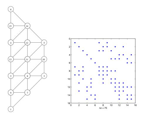
Figure 7.2: Unordered mesh and corresponding sparsity pattern.
